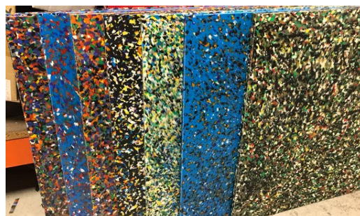
10mm Sheets produced on the C R Clarke R60 Sheet Press
